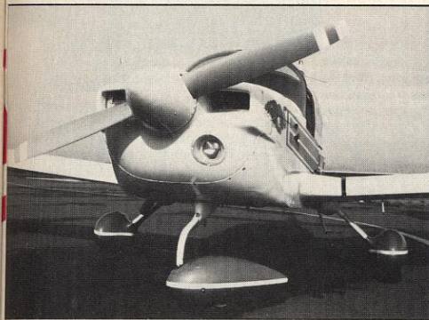
The original McCauley prop has an AD that requires its removal and inspection every 200 hours. However, there is an STC for a Sensenich prop that does away with the AD.
