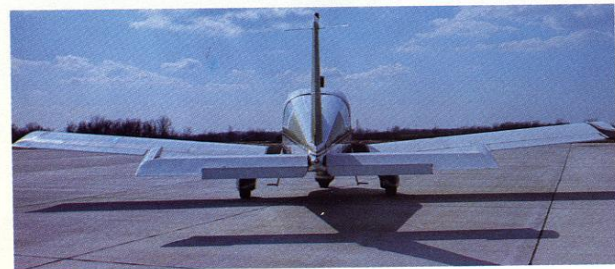
An aerodynamic clean-up and a Roy Lopresti redesigned empennage give Tigers near-retractable performance.
